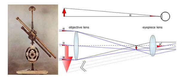
To construct a simple Galilean Telescope, all you really need is two convex lenses.
