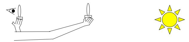
Finally, bring the lens at arms length in while holding the other lens near your eye until the distant object comes into focus.
